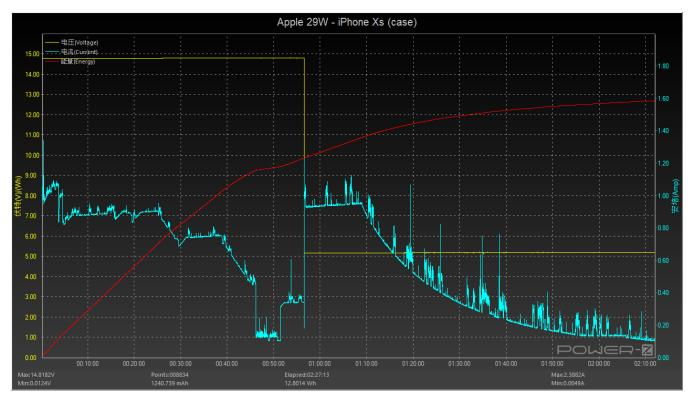
So during fast charge (~16W using Apple 29W USB PD charger) it is up to 10 minutes for extra cool down period observed at about ~70%. But overal charging time is still about 2h.
